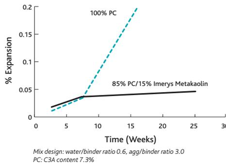
**FIGURE 2:** Deterioration of mortar bars immersed in sodium sulphate solution. PC contains 11 mass% C<sub>3</sub>A (Courtesy of the University of Glamorgan)
