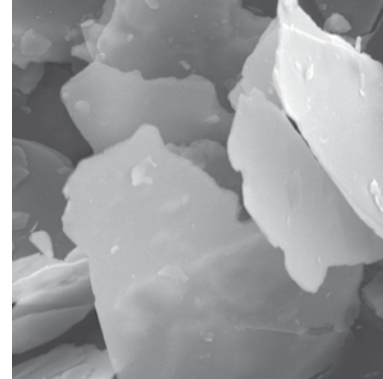
Right: SEM of Mica, demonstrating the large, platy characteristics that improves the performance of paints and coatings.
