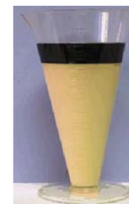
A real measurement of syneresis, an undesired effect in dextrin adhesive production.
